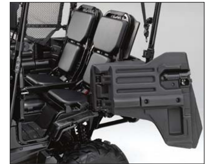
The two rear seats simply tilt up out of the bed structure with the release of a latch and lock into place, converting to five-person capabilities.
