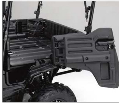
QuickFlip® seats can be quickly and easily converted from two-seat to three-seat or four-seat configurations and back to an open load-carrying bed without the use of tools and while retaining tilt function—an industry first.
