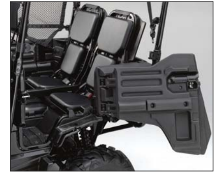
The two rear seats simply tilt up out of the bed structure with the release of a latch and lock into place, converting to four-person capabilities.
