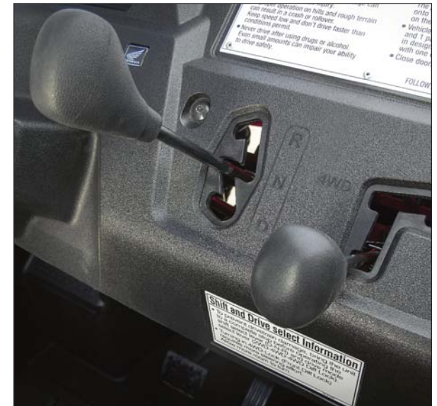
Selectable drive modes are full-time 2WD, 4WD and 4WD with front-wheel differential lock.
